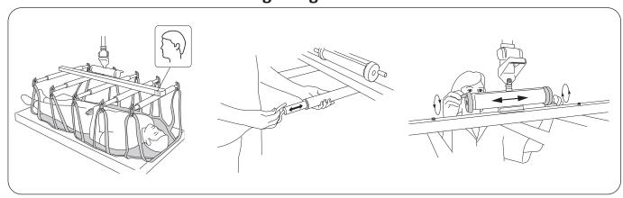
Remember that FlexoStretch<sup>TM</sup> accessory has a head end and a foot end. See the symbol for the head end [N]. Guide FlexoStretch accessory over the patient and lower it until it is about 50 cm above the bed. Connect the straps to the stretcher. Adjust the stretcher's width (70 cm to 95 cm) by pulling the lift arms out to a suitable position.
