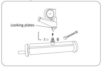
Likorall™ overhead lift (not R2R) and Golvo™ mobile lift FlexoStretch™ accessory is assembled using M10x25 screws and nuts directly into the lift's looking plates. Recommended tools: 6 mm Allen wrench and 17 mm closed-end wrench.
