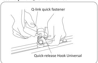
FlexoStretch accessory may be equipped with Quick-release Hook Universal (see page. 5) for simple and comfortable assembly into the lift without tools.
