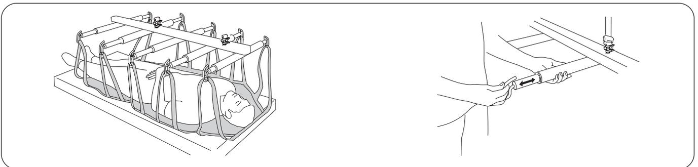
Move UltraStretch™ accessory over the patient and lower it. Hang all the strap loops on the stretcher. Note that the stretcher has a head end and a foot end. Adjust the stretcher width (70 to 95 cm, 27.6 to 37.4 inch.) by extending the liftarms to the appropriate length.
